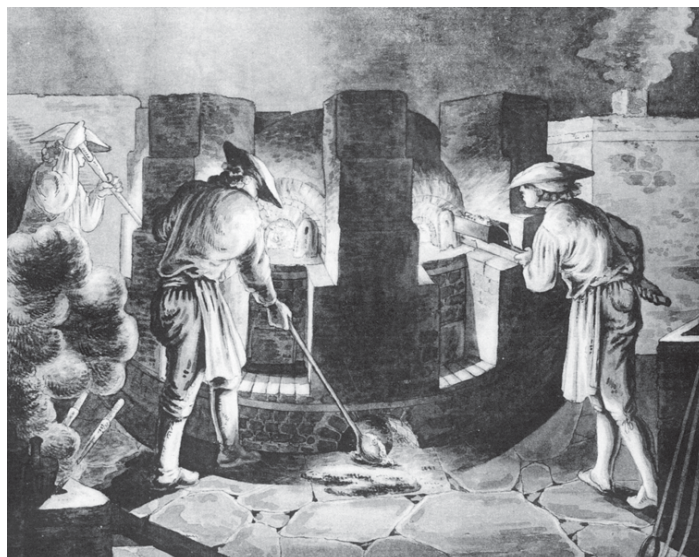
Figure 6- The hard work under the heat of the glass furnace. The melting of smalt was made in pots of clay at 1100 to 1250 ° C. The worker at right feeds the oven while at left the molten smalt is taken. Source of the engraving: Winckler, 1790 as reproduced by Hammer op. cit.
