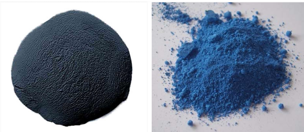
Figure 4. Left side, unrefined cobalt oxide (zaffre); right side the finished product (smalt) Image sources: left side [10], right side Wikimedia Commons, file “Cobalt Blue”- FK1954
