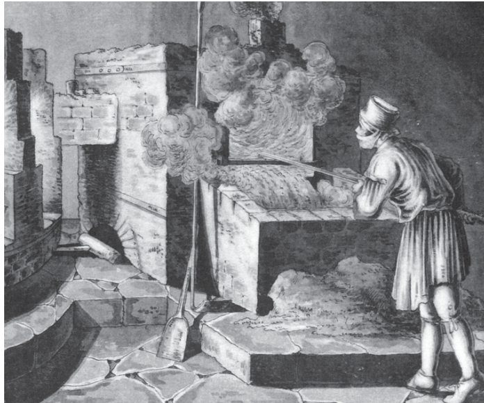
Figure 5- Roasting of the cobalt ore. Most of the unhealthy sulfur and arsenic fumes were channeled and condensed inside constructions called “smoke chambers” however the workers still had to cope with part of them. Source of the engraving: Winckler, 1790 [12] as reproduced by Hammer [11]
